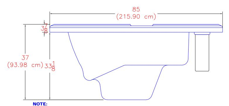
Dimensional tolerances are as follows due to variations in manufacturing: Length / Width / Height(s): +/- 3/8" Height Variance (side to side): +/-1/4"
