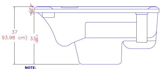
Dimensional tolerances are as follows due to variations in manufacturing: Length / Width / Height(s): +/- 3/8" Height Variance (side to side): +/-1/4"
