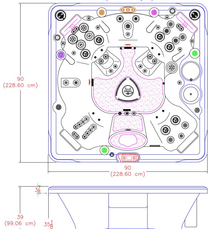
NOTE: Dimensional tolerances are as follows due to variations in manufacturing: Length / Width / Height(s): +/- 3/8"
